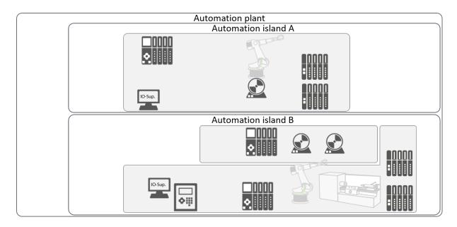
Figure 2-2: plant example with spatial and functional clustering
