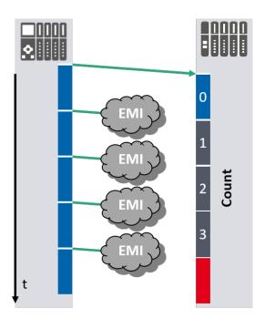
Figure 7-10: Communication problems with error threshold 3
