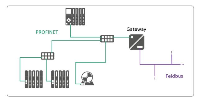
Figure 3-13: Use of a gateway to connect a fieldbus
