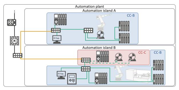
Figure 3-19: Plant example with complete topology
