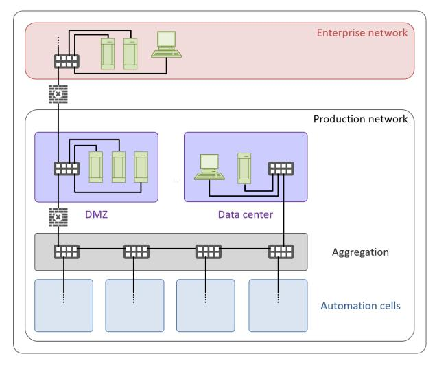
Figure 3-11: An example of a typical network architecture
