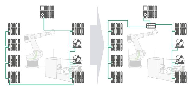
Figure 7-13: Example of reduced line depth
