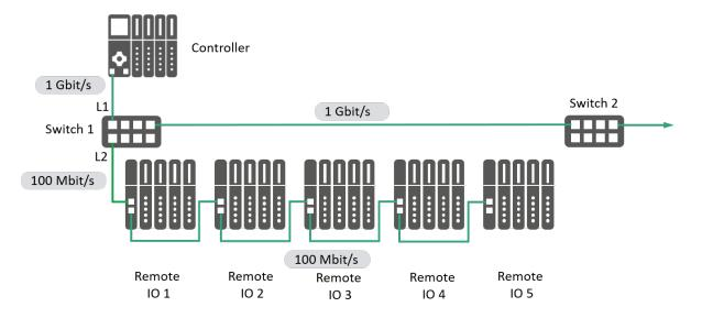
Figure 7-25: Example for input/output unbalanced link speed wise
