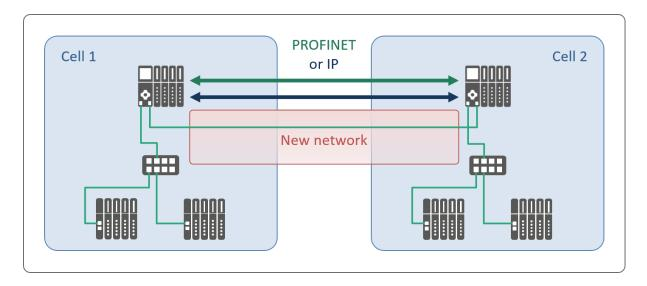
If devices have several Ethernet interfaces, these can be used to generate connections.
