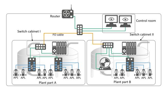
Figure 6-4: Example Plant Process Automation with Ethernet APL
