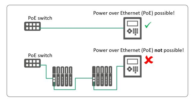
Figure 4-6: Topology limitations with Power over Ethernet
