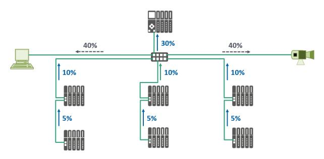
Figure 7-20: Optimized topology with reduced network load
