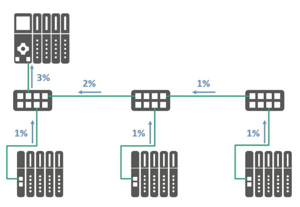
Figure 7-16: Example of network load distribution in a single controller application
