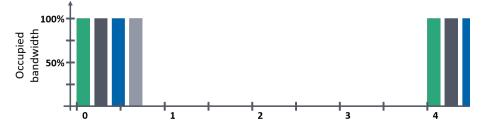
Figure 7-4: Network load, transmission cycle 4 ms, controller transmission clock 4 ms
