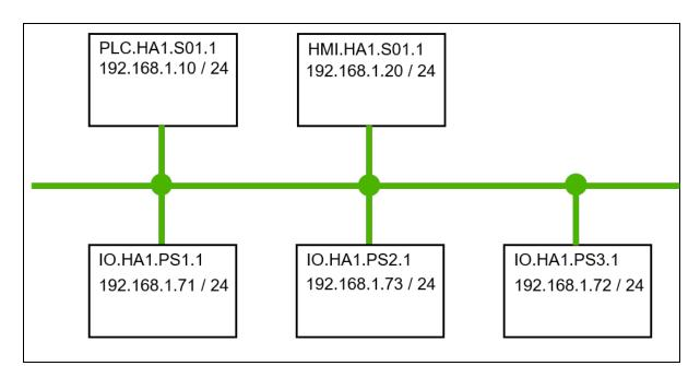
Figure 10-28: Example of PROFINET forwards documentation, logical topology plan
