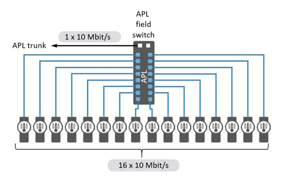
Figure 7-24: Example for input/output unbalance port count wise
