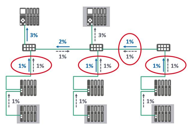
Figure 7-17: Example of network load distribution in a multi-controller application
