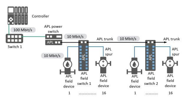
Figure 7-26: System Structure of an APL System with trunk and spur topology
