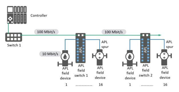
Figure 7-27: Ethernet-APL system with 100 Mbit/s industrial Ethernet to the field switches
