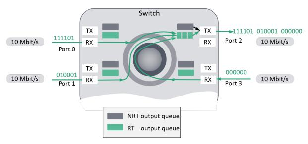
Figure 7-23: Congestion loss due to input/output unbalance port wise
