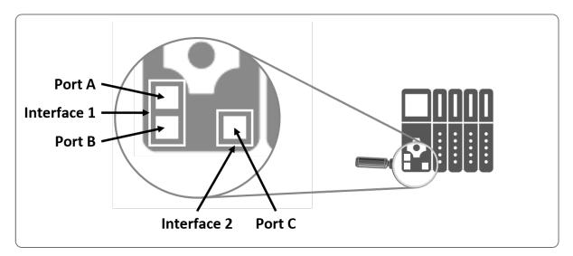
Figure 3-1: Difference between the terms port and interface
