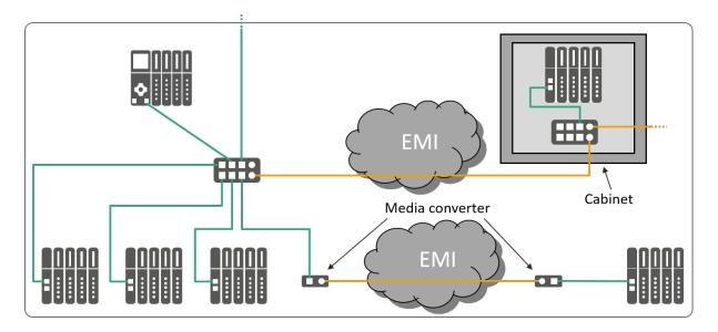
Figure 3-9: Application of optical fiber technology for EMI
