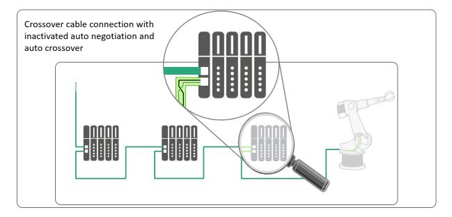
Figure 4-7: Implementation of "Fast Startup" with PROFINET
