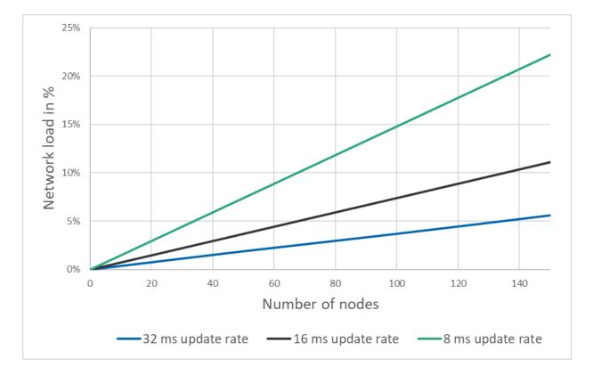
Figure 7-9: Cyclic PROFINET network load as a function of update time and number of network nodes (typ. PROFINET packets) at 100 Mbit/s data rate
