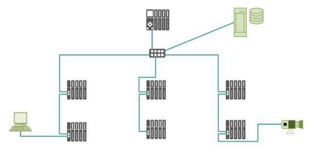
Figure 7-18: Example topology with standard Ethernet nodes
