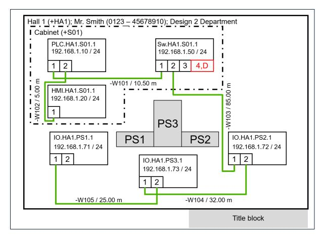
Figure 10-27: Example of PROFINET forwards documentation, physical topology plan
