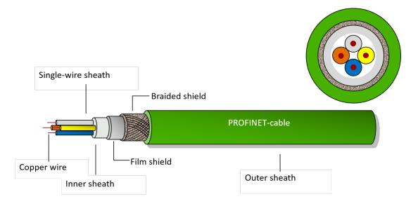
Figure 10-1: PROFINET cable type A
