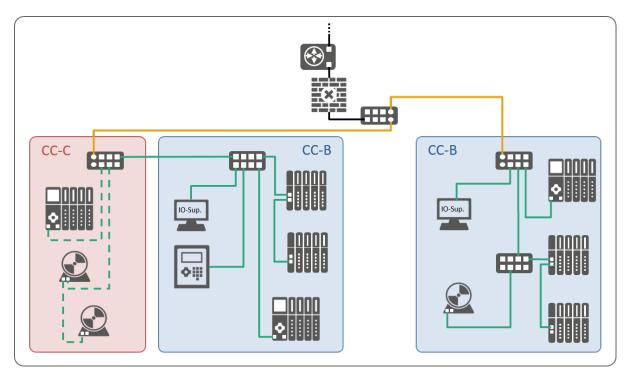
Figure 3-20: The plant example from network perspective
