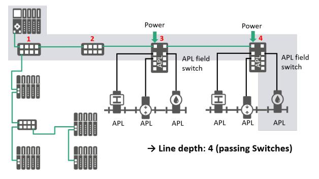
Figure 7-14: Line depth with APL Field-switches connected to 100 Mbit/s network
