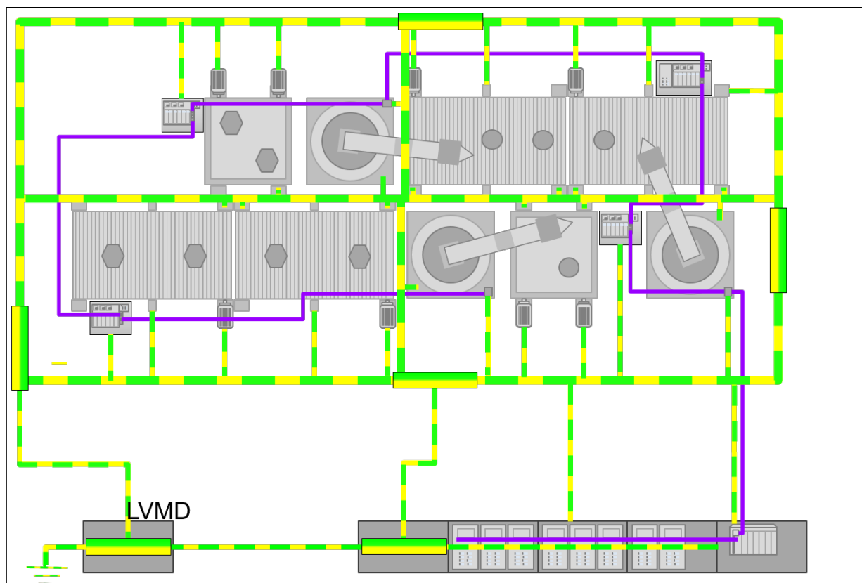
Figure 4.32: Stubs of the meshed equipotential bonding system
