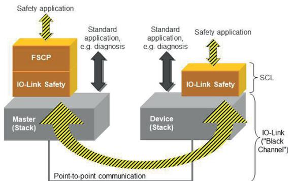
Fig. 5: “Black Channel” principle
